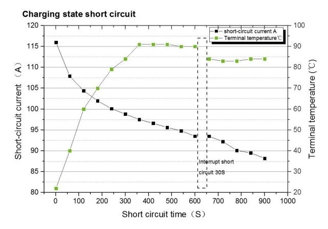
Resistance of the wire was 2 m $\Omega$  in the short circuit. Neither fire nor explosion, or any battery deformation occurred during short circuit test.
