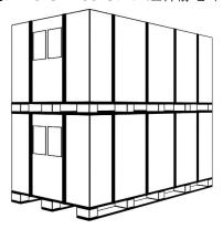
3.4.2 Normal warehouse storage (moisture < 85% and temperature in the range from -20°C to + 50 °C): Be stacked no more than two layers.
