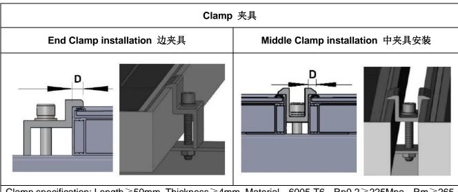
Clamp specification: Length ≥50mm, Thickness ≥4mm, Material: 6005-T6, Rp0.2 ≥ 225Mpa, Rm ≥ 265 MPa
