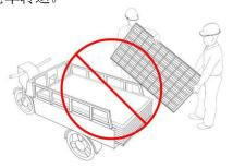
3.3.6 No handling the module with rope.
