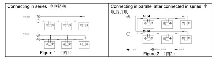
The number of modules in series and in parallel shall be designed reasonably according to the system configuration.
