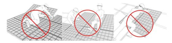
Do NOT damage or scratch the front or backside surfaces of the module.
